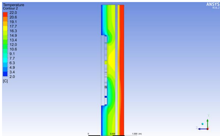
FIGURE 81: TEMPERATURE FIELD WHEN THE AHU IS SWITCHED ON
