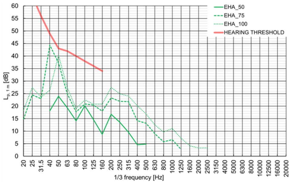
FIGURE 149: 1/3 SPECTRUM OF SOUND PRESSURE LEVEL AT A DISTANCE 1 M FROM EHA FOR PROTOTYPE_1.
