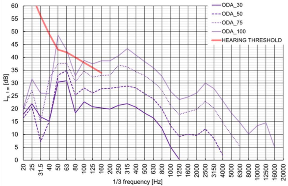
FIGURE 144: 1/3 SPECTRUM OF SOUND PRESSURE LEVEL AT A DISTANCE 1 M FROM ODA FOR PROTOTYPE_2.
