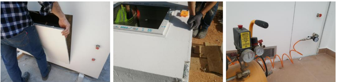
FIGURE 6: (LEFT): ACCESS PANEL OPERATIONAL TEST, (MIDDLE): TRANSPORTATION HINGES TEST, (RIGHT): PIPEWORK AIR PRESSURE LEAKAGE TEST.
