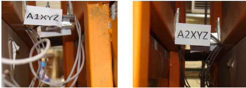
FIGURE 107: INSTRUMENTATION SET-UP: ACCELEROMETERS PLACED AT MEASUREMENT POINTS A1 AND A2 (SMARTWALL)
