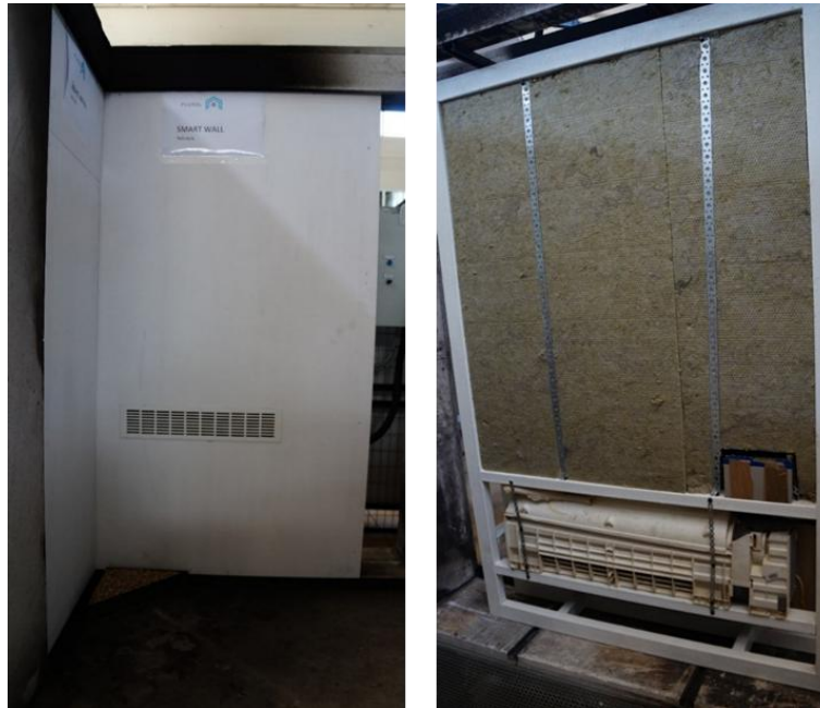
FIGURE 41: SMARTWALL WITH FAN COIL AND BATTERY, EXPOSED SIDE (LEFT) AND UNEXPOSED SIDE (RIGHT).
