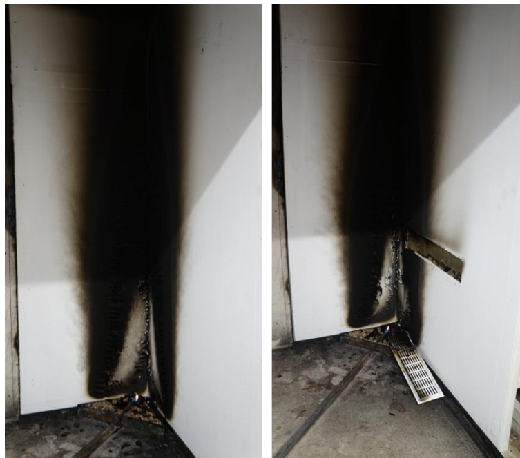
FIGURE 43: SMARTWALL WITHOUT (LEFT) AND WITH FAN-COIL AND BATTERY (RIGHT) AFTER THE TEST.
