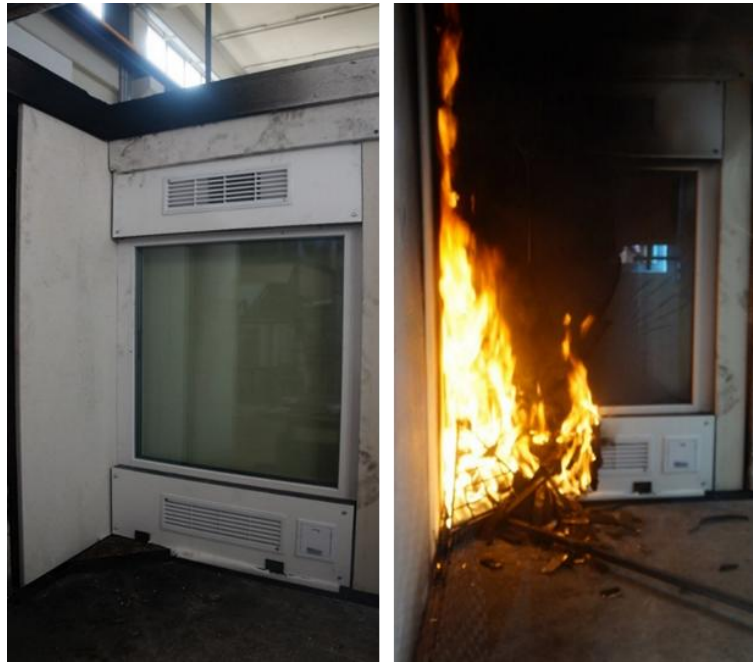
FIGURE 44: SMART WINDOW CONFIGURATION BEFORE (LEFT) AND DURING (RIGHT) THE FIRE TEST.
