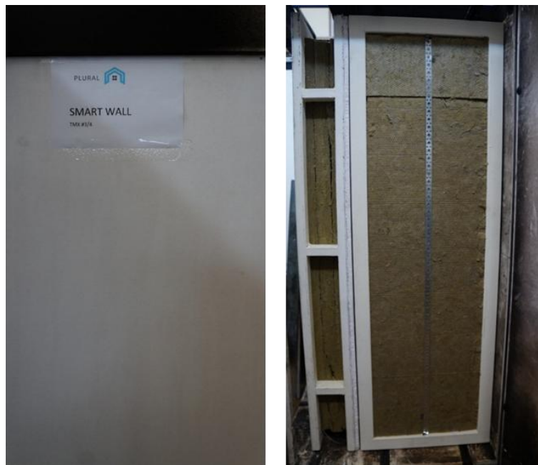
FIGURE 40: SMARTWALL WITHOUT FAN COIL AND BATTERY, EXPOSED SIDE (LEFT) AND UNEXPOSED SIDE (RIGHT).
