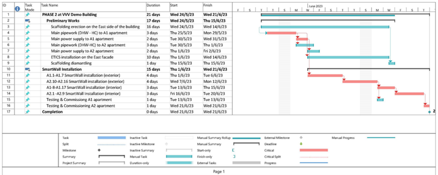
FIGURE 4: PHASE 2 – INSTALLATION OF SMARTWALL SYSTEMS
