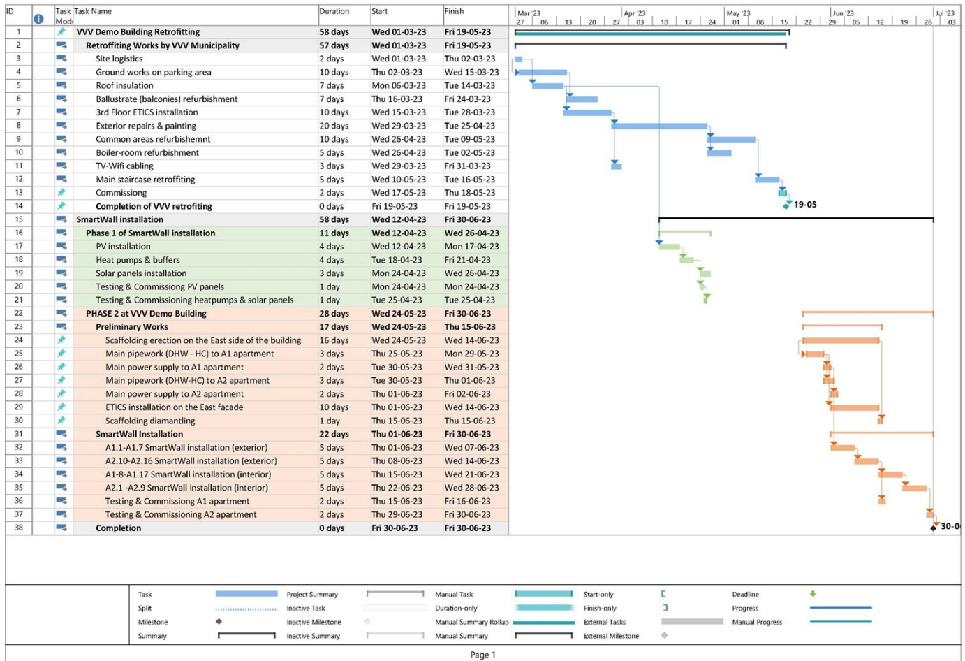
FIGURE 2: OVERALL CONSTRUCTION SCHEDULE FOR VVV RENOVATION
