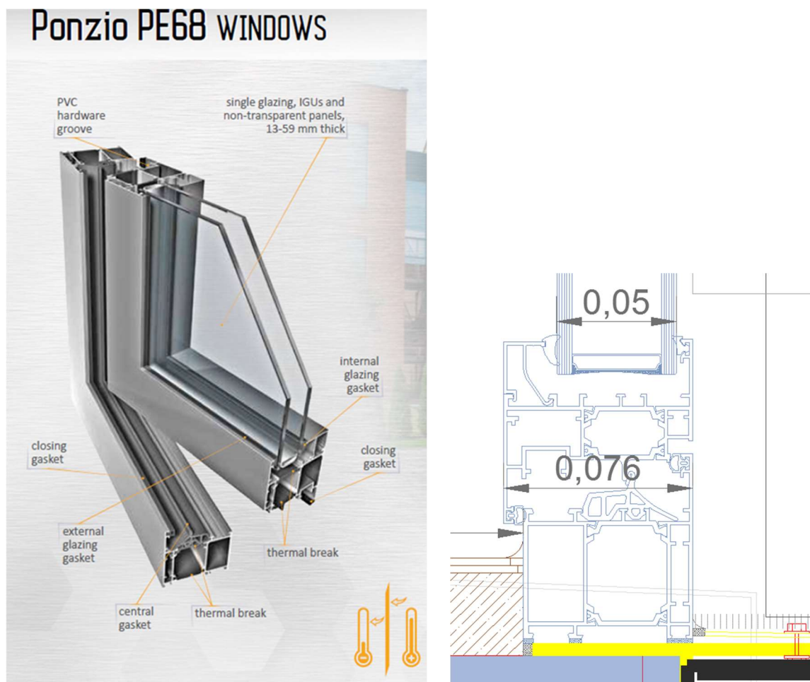
FIGURE 3.1-1 WINDOW SOLUTION FOR TERRASSA DEMO
