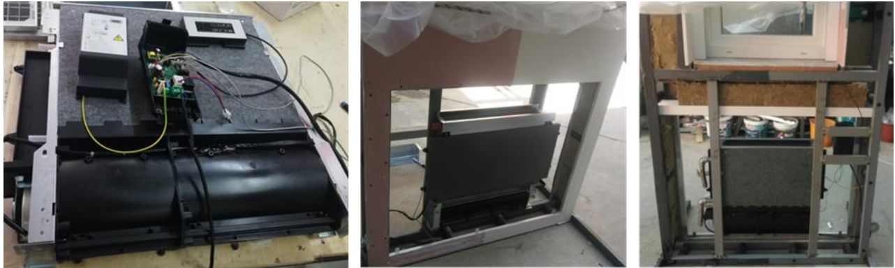
FIGURE 3.3: THE FWXM10ATV3 FAN COIL MODEL DURING THE ASSEMBLY OF ONE OF THE PROTOTYPES
