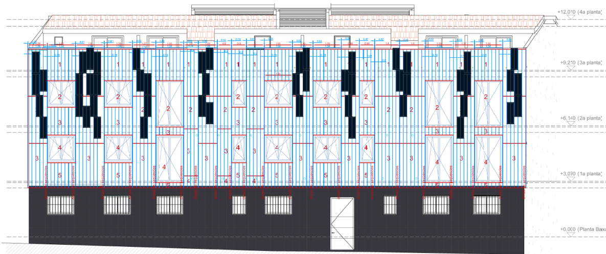
FIGURE 40: INTEGRATION OF PVs IN THE FACADE
