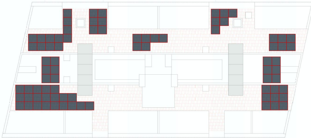
FIGURE 41: INTEGRATION OF PVs IN THE ROOF
