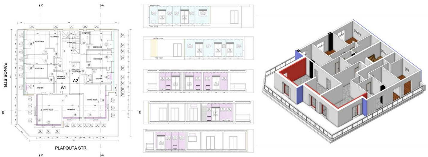
FIGURE 59: INTEGRATION AND POSITIONING OF SMARTWALL PANELS IN GREEK DEMO SITE
