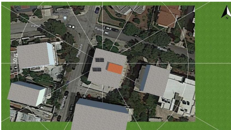
FIGURE 68: OVERHEAD VIEW OF PV ARRAYS – PROPOSED POSITIONING
