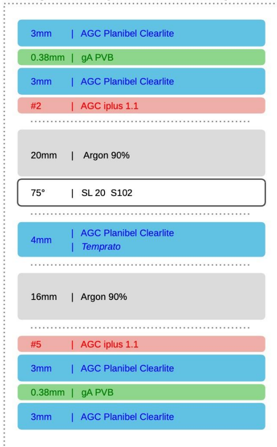
FIGURE 9 GLAZING CONFIGURATION AND A SAMPLE OF THE GLASS WITH INTEGRATED SHADING SYSTEM.
