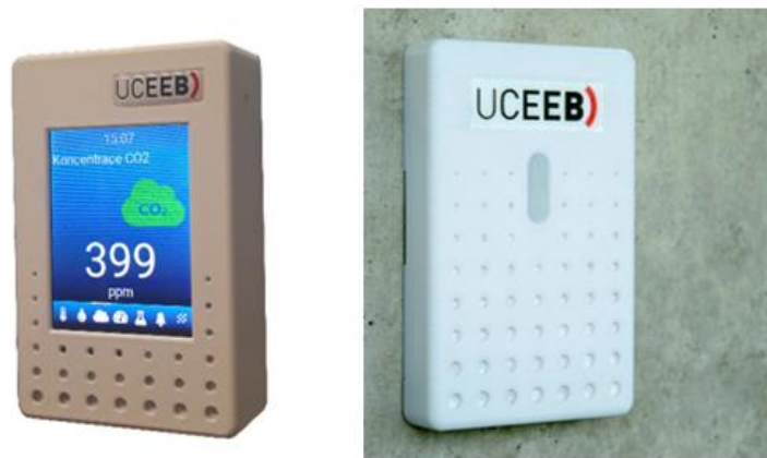
FIGURE 8 CVUT IEQ SENSOR PLATFORM TO MONITOR INDOOR AIR QUALITY AND BUILDING TECHNOLOGIES
